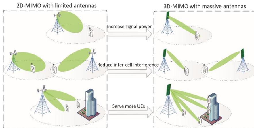
**Figure 2-1** Technical principles of Massive MIMO
