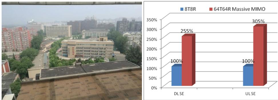
Figure 3-2 Spectrum efficiency improvement in campus scenario
